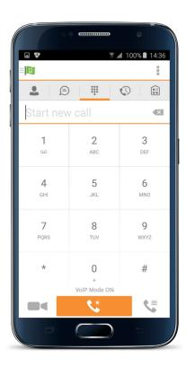
The Dial Pad tab displays a dial pad and a text field used to enter numbers. The dial pad is one of the options used to make audio or video calls. There are three buttons below the dial pad: Call, Video call, and Dial pad menu that are configurable by the service provider. The top text field also has a delete button that, when pressed, deletes one character at a time.
